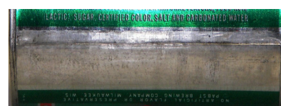
Notice the bottom edge overlaps the top edge creating an uneven finish
